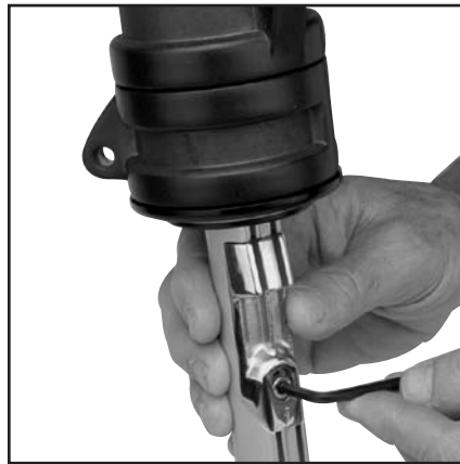
Loosen screw one revolution only .
