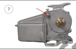
Place the pawl assembly from previous step on the top M10 thread. Tighten it and secure it in place.
