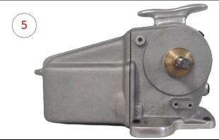
Place the rope kit's inner cone clutch on the shaft. It is advised to use yellow marine grease on the cone clutch surface that is in contact with the gypsy.
