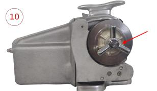
Place on the shaft the stock outer cone clutch and the stock tripod. It is advised to use yellow marine grease on the cone clutch surface that is in contact with the gypsy.
