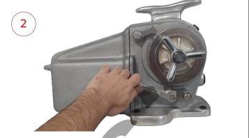
Remove the stripper by unscrewing the two M8 screws.
