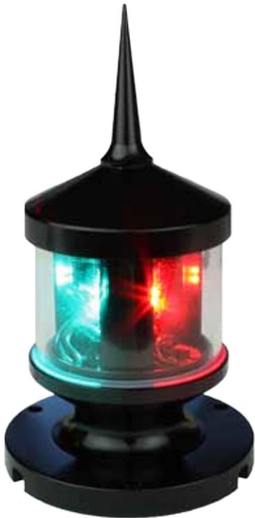
Lunasea's Tri-color/Anchor/Flash and Anchor/Flash LED navigation models have the added features that you asked for, and more. This lightweight fixture, made of machined aluminum weighs just 140 grams (4.9 ounces). We've added emergency flash, auto daylight turnoff for anchor, and a removable bird spike. The waterproof connector is only 0.38 inch wide for easier cable routing. The glass lens assures excellent light transmission for the life off the product. 3 year warranty.
