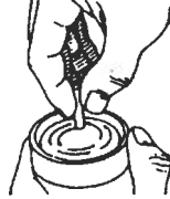
Starting in the center of the lens, gently rub in a circular motion from the center to the outside.
