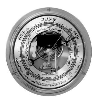
**Installation:** The barometer is attached to the wall, or a wooden plaque if desired, using the three brass wood screws enclosed. Before mounting, the movement should be set to compensate for your altitude by turning the set-screw on the back with a small screw driver. The barometer is set at the factory for the reading at sea level, so if you are located at or slightly above (<100 feet) sea level, little or no adjustment should be necessary.
